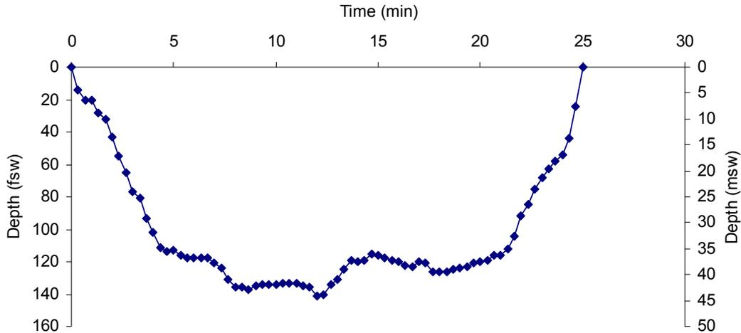
Figure 2.5.1-2 Dive profile containing rapid ascent and omitted decompression
